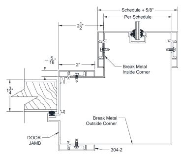
Note: This configuration must be reinforced on site.
