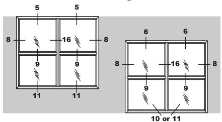
**Note:** The stud at detail 6 and 8 must be inverted so that the glass pocket will clear. If installing to ceiling grid, (Detail 5), ensure that the ceiling grid is level and that the head channel is level and square before installation of frame and glazing material.
