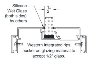
219 series has an expanded pocket and uses standard vinyl with 1/2" glass.
